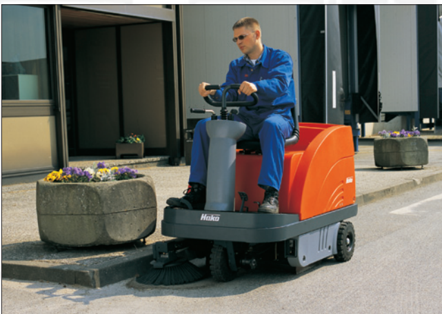
Hako-Jonas 900 V: For outdoor applications with hydrostatic drive and rpm regulated petrol engine.
